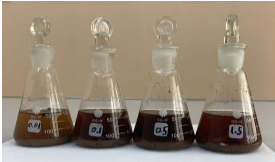
Figure 8. Sorbents activated by NaOH with concentrations from 0.01 to 1.5 mol/L
