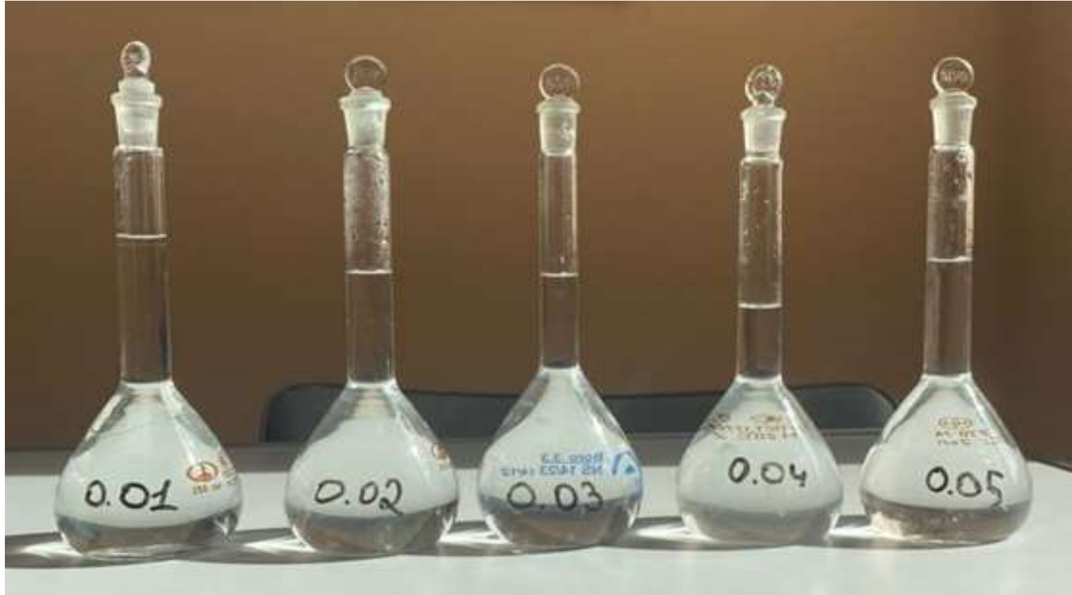
Figure 2. Preparation of model solutions with a concentration of zinc (0.01-0.05 mol/L)
