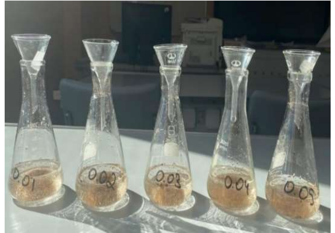
Figure 7. Filtration of model solutions using each sorbent
